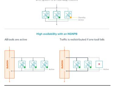
Figure 2-2: An N+1 configuration for redundancy vs. using load balancing for high availability.
