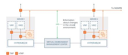
**Figure 4-3**: The NGNPB is integrated with the management center of the virtual platform so it can react automatically to dynamic changes in the number and location of the VMs.
