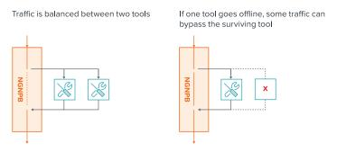
**Figure 2-4**: Logical bypass can also address a load balancing situation where one tool goes down by preventing the surviving tool(s) from being overwhelmed.
