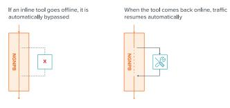
**Figure 2-3**: Logical bypass: when an inline security tool goes offline, the NGNPB senses the outage and keeps network traffic flowing around the tool.
