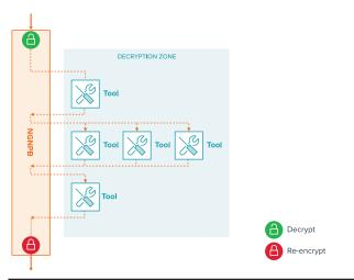
**Figure 3-2**: An NGNPB creates a decryption zone where tools have visibility into all decrypted traffic and decryption is performed once with no impact on the performance of the tools.
