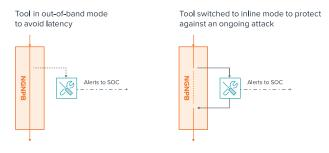
Figure 2-5: NGNPBs can switch tools from out-of-band to inline mode during an attack.
