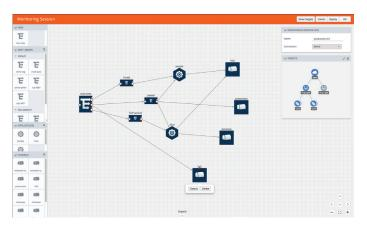
**Figure 4-6**: The NGNPB orchestration and management module can manage policies for monitoring network traffic on the cloud platform. (Source: Gigamon)
