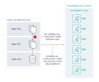
Figure 4-4: The enterprise can't put TAPs or SPAN ports in the cloud platform to monitor traffic between the application tiers.
