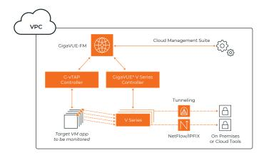
**Figure 4.** GigaVUE Cloud Suite for AWS VMs is composed of five components: G-vTAP, G-vTAP Controller, V Series, V Series Proxy (optional), and GigaVUE-FM.
