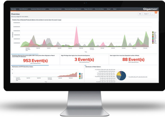
Figure 3. Gigamon AMI dashboard within Splunk, showing suspicious connections, unusual login activity, HTTP error codes and more.
