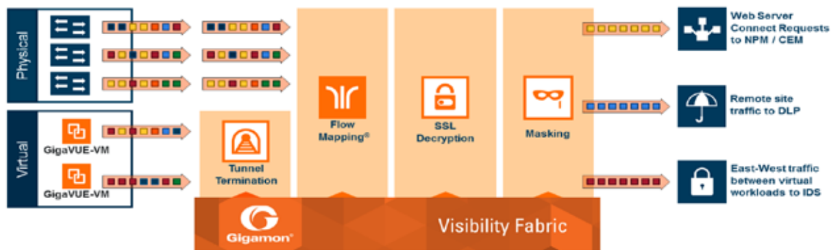
Figure 18: Sample GigaSMART Service Chaining
