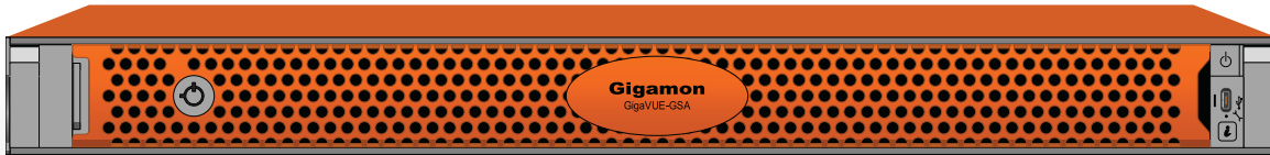
Figure 1. The GigaSMART appliance scales GigaSMART processing and metadata delivery in a compact single-rack-unit design.
