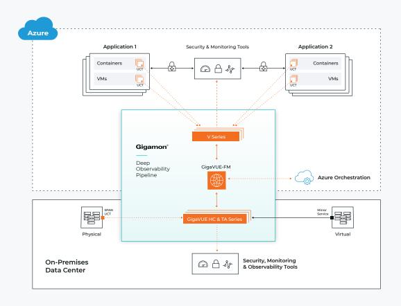
Figure 1. The Gigamon Deep Observability Pipeline acquires, processes, and forwards traffic within an Azure VNet.
