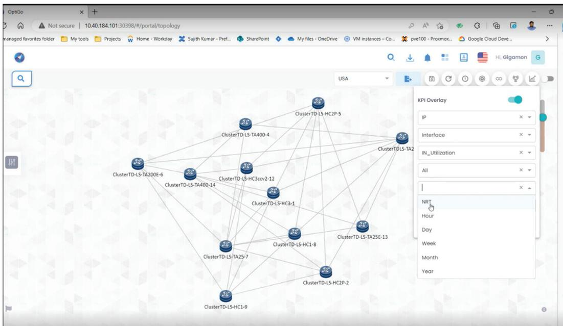
Finally, fault management data can be implemented and displayed for devices to show network device system alarms. Correlation of fault management data from disparate devices can eliminate alarms and generate incidents to reduce the mean time to detect (MTTD) issues. Then, performance KPIs can be overlaid for interfaces in between network devices to show network performance health:
